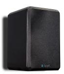
Apart VINCI Series has been expanded with a new VINCI4-16 bass reflex cabinet loudspeaker. VINCI4-16 has an impedance of 16 ohms, what allows the connection of up to 4 VINCI4-16 loudspeakers in parallel on a single amplifier channel, capable of handling a 4 ohm load.
